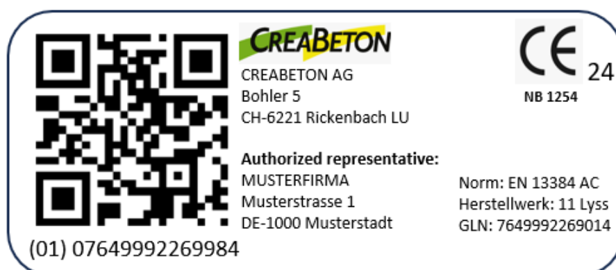
Figure 3: Possible representation of a label with the required DPP components. Source: Creabeton AG (type plate) and NexSwiss (DPP behind the QR code)
